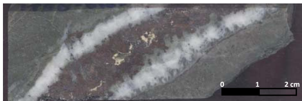
Figure 3. Photograph of drillcore showing a zoned mineralized veinlet cross-cutting the andesitic host rock.
